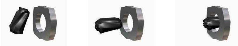
After passing through the filter, the long particle will be carried by the water jet to the orifice and will obstruct it.
